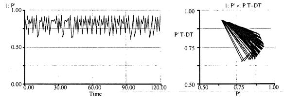
Alternative values of W result in damped oscillations, oscillations with one, two and higher periods, and ultimately chaos which is shown in the two figures above. Despite the simplicity in its assumptions, the model exhibits a wide range of behaviors that vividly
