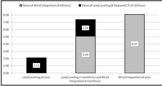
Figure 15. Summary GCAES values, with the middle case showing over \$7 billion in value due to a combination of load leveling, reduced CTs and wind integration.
