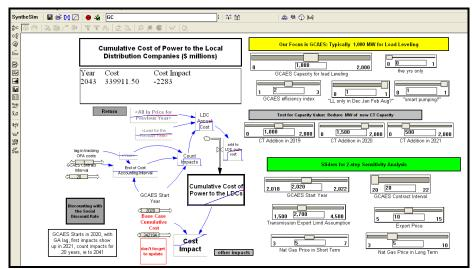
Figure 14. Value to the Load Distribution Companies from the use of 1,000 MW of GCAES for a combination of load leveling (energy arbitrage) and displacement of new CT units.
