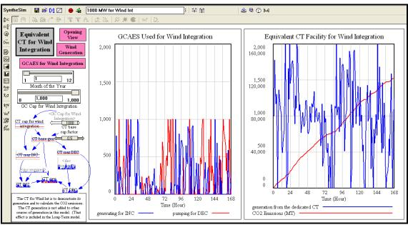
Figure 13. Wind integration results with a 1,000 MW GCAES (on the left) and a 2,000 MW CT facility (on the right).
