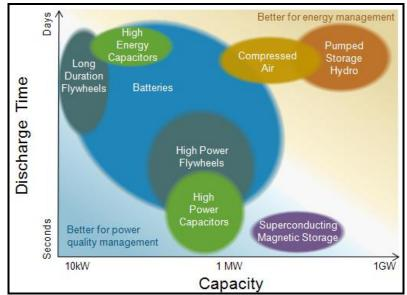
Figure 1. Classification of electricity storage technologies (EIA 2013).
