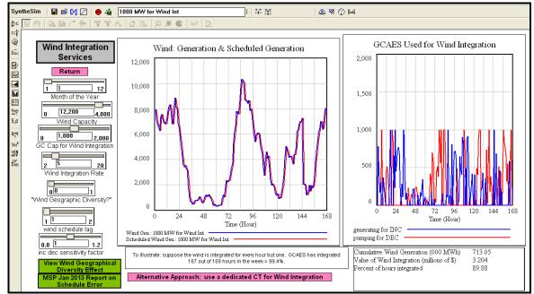
Figure 12. Results from application of 1,000 MW of GCAES toward wind integration during a typical week of January of 2028.
